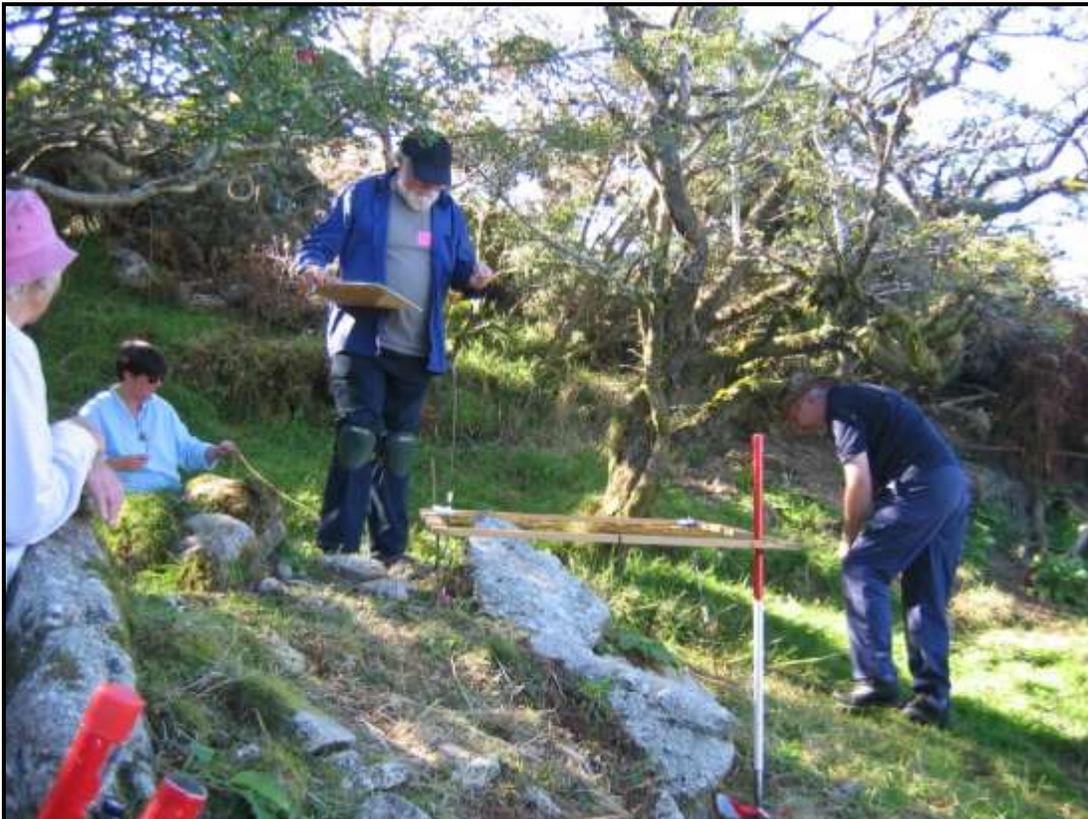
*Figure 6. Details were added to the survey using planning frames.*
