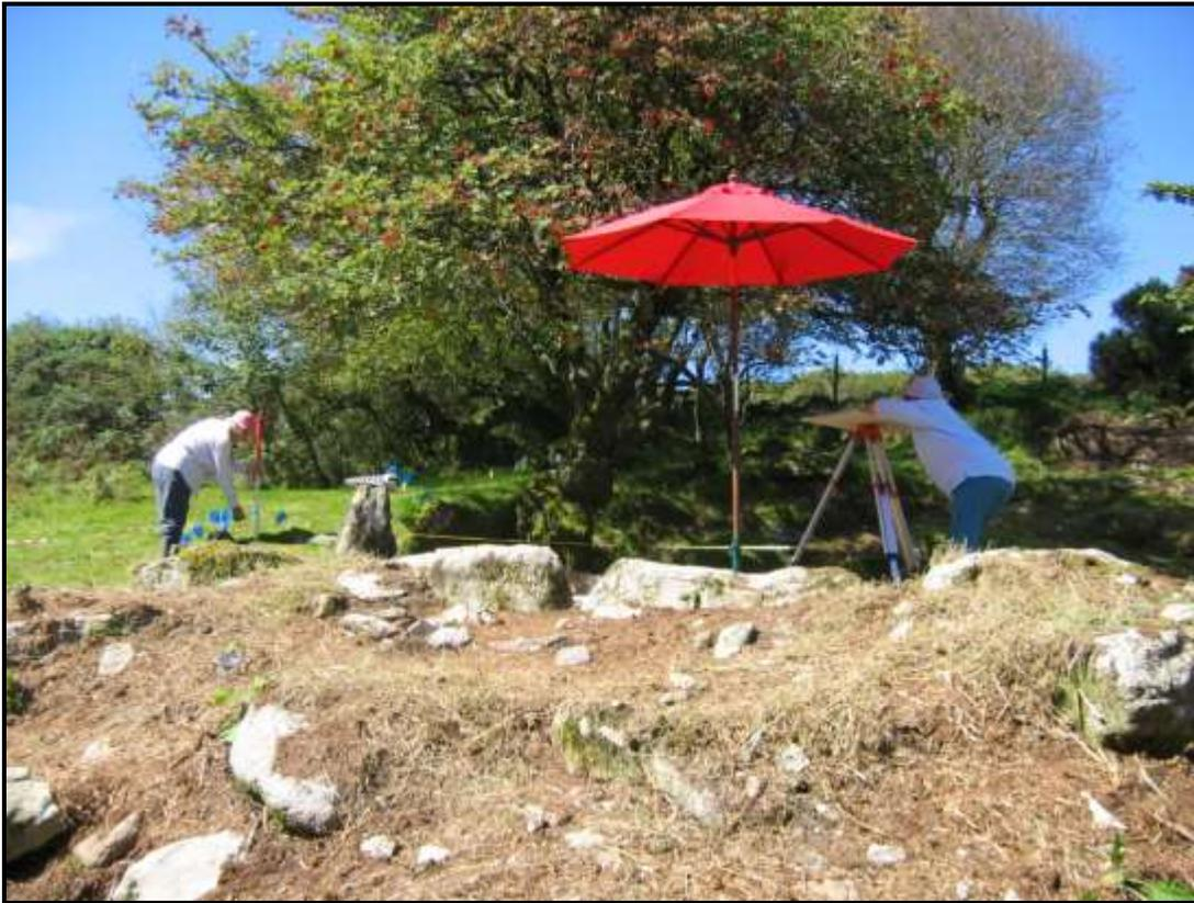
*Figure 5. The main part of the survey was carried out using planetables at a scale of 1:50.*
